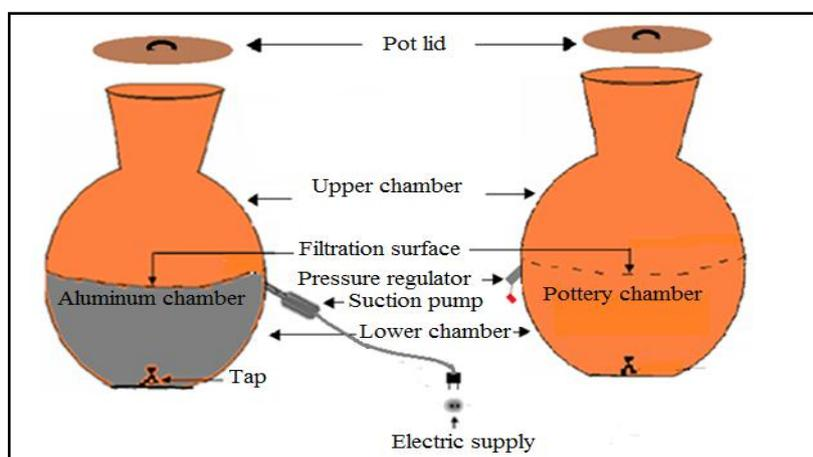
Figure 2. External views of the hypothesized models of the water pot.
