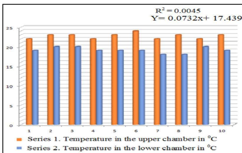
Figure 8. Drop in temperature of water in the lower chamber of the modified pottery pot.
