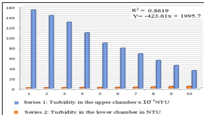
Figure 4. Efficiency of the modified pottery pots for reduction of water turbidity.
