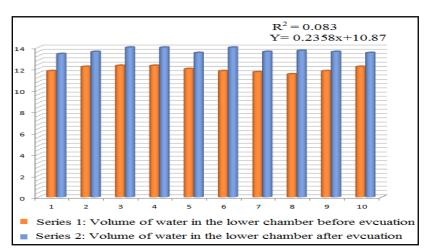
Figure 7. Productivity levels of filtered water attained by the modified model before and after evacuation.
