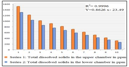
Figure 6. Efficiency of the modified pottery pots for reduction of the total dissolved solids.
